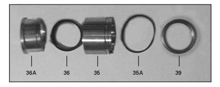
12. Lubricate weep seal (36). Place, weep seal (36), and pressure ring (36A) into the seal sleeve (35). Assemble the o-ring (35A) onto seal sleeve and lubricate.
